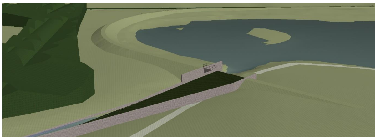
Figure 4-2: Option 2 Tymon flood storage embankment
